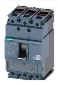
CIRCUIT BREAKER 3VA1 IEC FRAME 160 BREAKING CAPACITY CLASS S ICU=36KA @ 415 V 3-POLE, LINE PROTECTION TM240, ATAM, IN=40A OVERLOAD PROTECTION IR=28A ...40A SHORT CIRCUIT PROTECTION II=5...10 X IN CABLE CONNECTION
